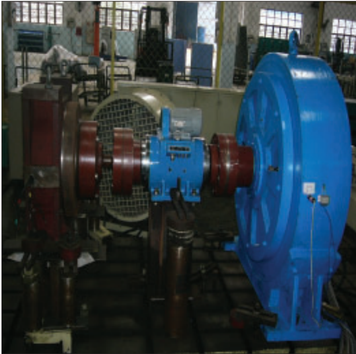
ACPM machine load testing
