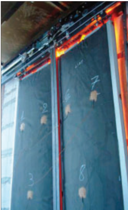
Figure 4: A Wittur Hydra two-panel center-opening door during testing for EN 81-55 EI 120 certification.
