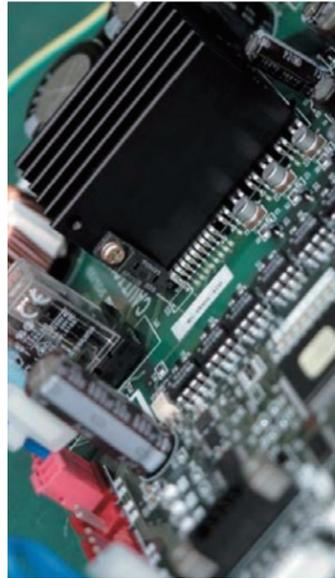
An elevator operation system with multiple microcomputers makes maximum use of a "Distributed Control System." Hall indicators, car operating boards, and control panels incorporate high-performance microcomputers. These independent microcomputers analyze elevator operating conditions utilizing self-diagnostic functions and implement immediate control of elevator operations. Also, data transmission buses between microcomputers increase data processing capability.
